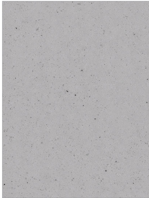
Residual particles on the filter membrane Microscope: Axio Imager 2, objective: EC Epiplan-NEOFLUAR 10x/0.25
